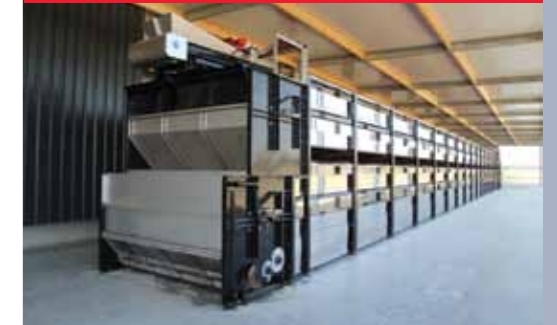
Manure drying with ventilation air from the poultry house
